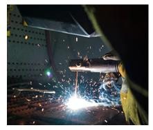
Selecting a quality MIG wire is critical. It can be more forgiving and produce a sound weld even under less than perfect conditions. Take, for instance, a plate with surface contaminants. The right MIG wire for that application may make some pre-welding operations obsolete. And, as more companies move to robotics, a quality MIG wire will provide accuracy in wire placement and consistency in the weld, making rework less of an issue.
