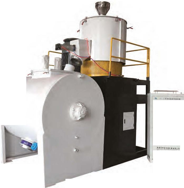
Hot and cold seal feature silicone rubber seal with reliable and deformation-free sealing effect even at high temperatures.
