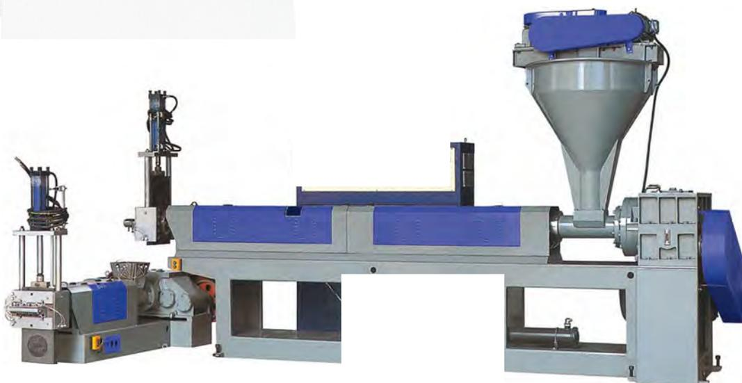
Various models available. Production between 200 and 400 kg / h. Maximum dimensions 5x2.6x 14 m. Maximum weight 9,200 kg.
