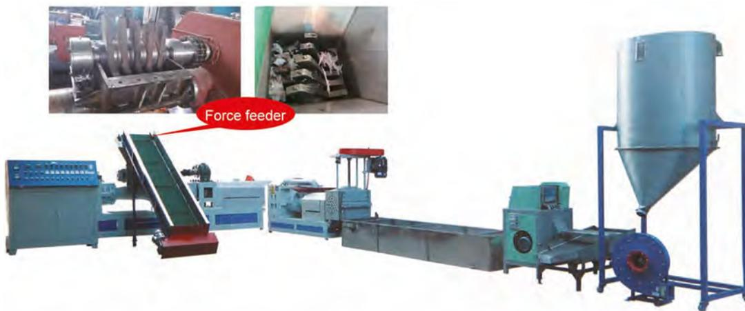
Depending on the model, this granulation line, made up of three stages, is capable of processing between 180 and 800 kg / hour.
