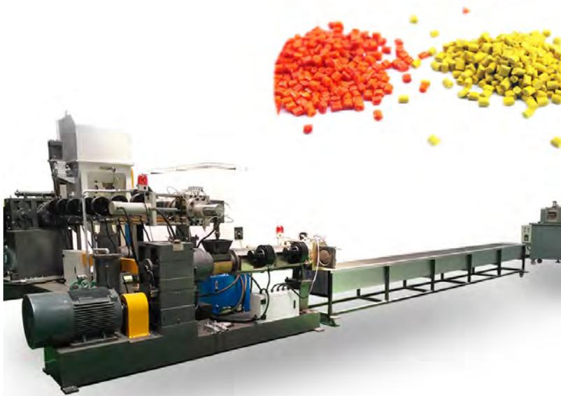
Equipment specialized in the granulation of POLYPROPYLENE (PP) and POLYETHYLENE (PE) flakes.
