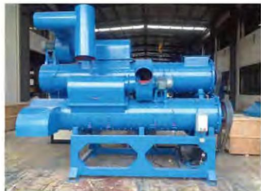
The tag remover can be divided into two categories: one-axis tag remover, three-axis tag remover. They can remove the plastic tag using air suction and friction from the blade. Single axis tag remover can remove the tag by 95% and 100% removal ratio with large capacity by three axis tag remover.
