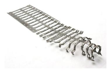
Progressive die stamping is a process very cost-effective and widely used for mass production of stamped parts which require complicated in-press operations manufacture, because it can be completely automated and have a high dimensional accuracy. It is specially used to produce large series of small and medium parts.
